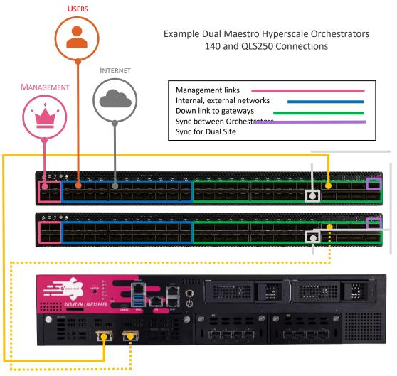
The QLS250 Maestro package includes the Hyperscale Orchestrator 140 model with 48x 10GbE, 8x 100GbE ports and a total fabric capacity of 1.2 Tbps. For redundancy, deploy two Orchestrators of the same model together.
