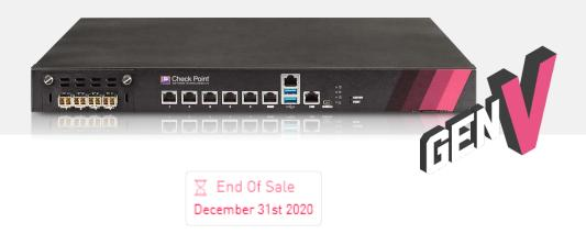
Check Point's 5200 Next Generation Firewall offers a fully integrated, unified solution tuned to deliver maximum security against 5th generation threats without compromising performance. 5200 Security Gateway provides the most advanced threat prevention security for demanding enterprise networks.
