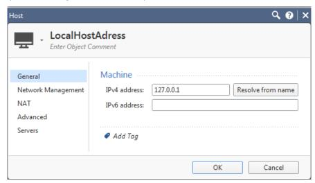
Enable the ID Awareness Web API and add the local host object to access object to the allowed hosts. This configuration step allows the PDP Broker process accessing the ID Awareness API.
