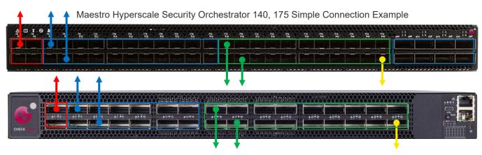
The Hyperscale Orchestrator 140 is a mid-range model with 48x 10/25GbE and 8x 40/100 GbE ports with a total fabric capacity of 1.28 Tbps. The Hyperscale Orchestrator 175 is a high-end model with 32x 40/100 GbE ports and a total fabric capacity of 3.2 Tbps.
