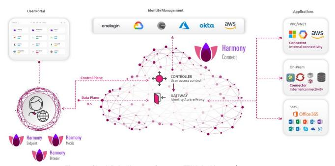
Figure 2: Check Point Harmony Connect - ZTNA Architecture<sup>1</sup>
