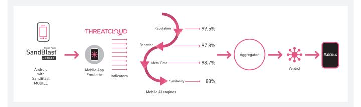
SandBlast Mobile uploads every installed application to the cloud for evaluation. In the cloud, several engines are inspecting the application; some of them based on Al. Each of the Al models calculates the probability of the application to be malicious. The aggregator model decides, based on those probabilities, and a pre-defined threshold, whether the application is malicious, risky or benign. In this case, the application was successfully identified as malicious.
