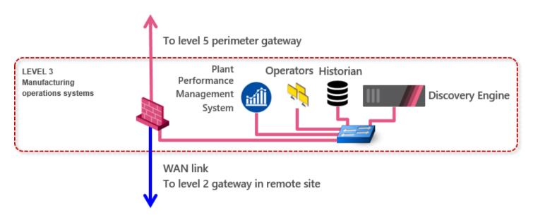
The security gateway in level 3 segments the IT from the OT part of the network and micro-segments level 3 itself. The plant management system, the operators, and the historian should all go in separate VLANs, while the gateway controls who is allowed to talk to who.
