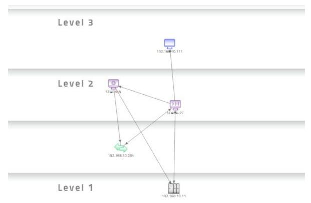
A second screenshot from the Claroty console showing where the discovered devices are situated according to the Purdue model.
