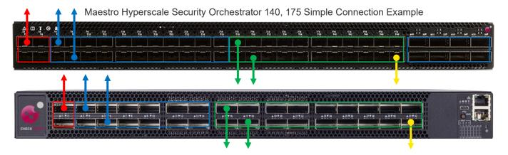
The Hyperscale Orchestrator 140 is a mid-range model with 48x 10GbE and 8x 100 GbE ports with a total fabric capacity of 1.28 Tbps. The Hyperscale Orchestrator 175 is a high-end model with 32x 100 GbE ports and a total fabric capacity of 3.2 Tbps.
