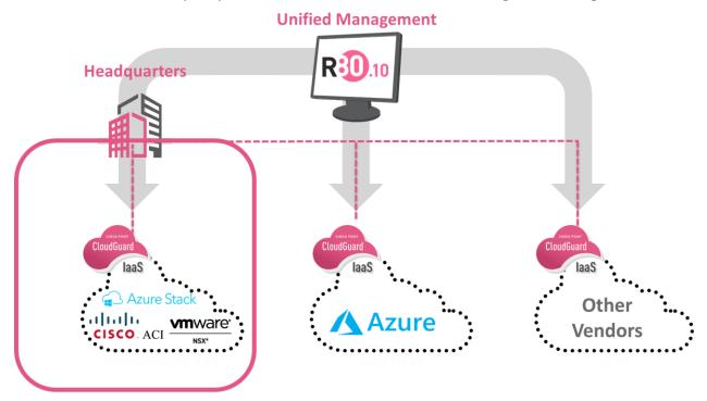
Management server location is completely flexible and can be located anywhere across the environment. It is also possible to setup the management server in high availability mode across platforms (e.g. primary management located on premises with a backup server located in a location designated for disaster recovery).
