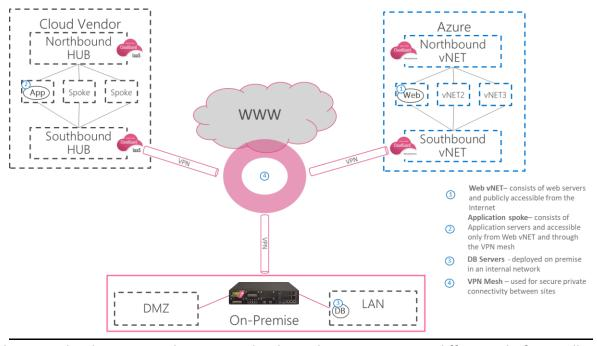
As shown in the diagram, implementing CloudGuard gateways across different platforms allows us to both control traffic in each location specifically but also enforce our security policy across and between locations.
